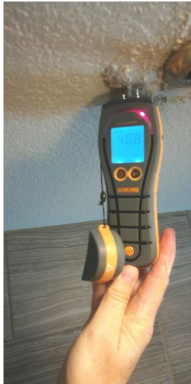
40% moisture, 15% would be normal. Mold grows above 20%
