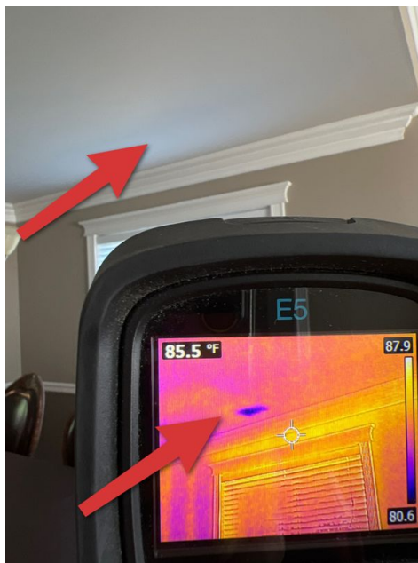
Infrared image of cold spot
