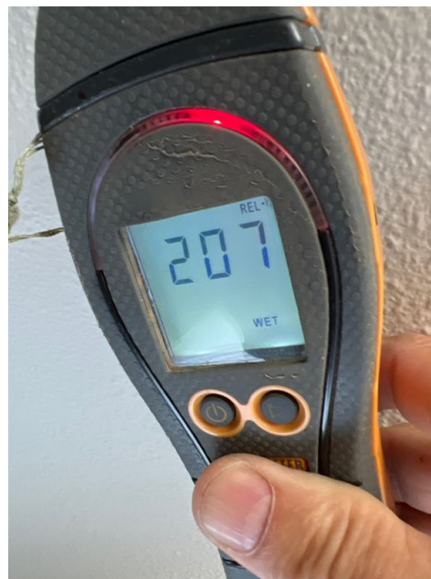
Above 20% moisture reading detected
